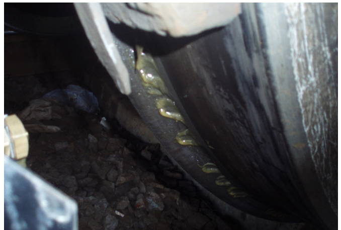
Lubricant is applied to the wheel flange
