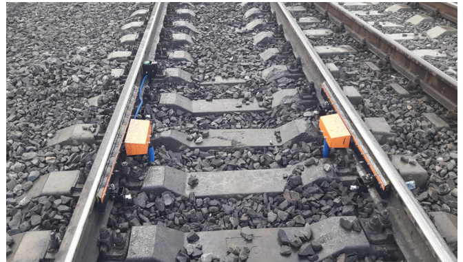
Lubricant is delivered through twelve channels on each of the lubrication bars.
